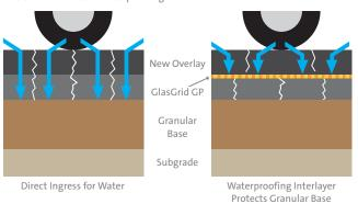
GlasGrid GP can be installed with traditional asphalt binders and requires 25% less hot asphalt cement to be saturated. Compared to traditional non-wovens, GlasGrid GP reduces your project's system costs as well as its carbon footprint.
